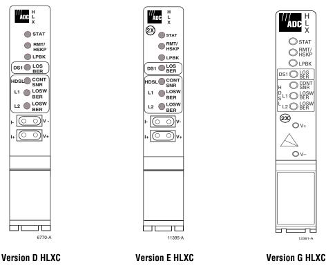
Figure 572-1. HLXC Module Front Panels
